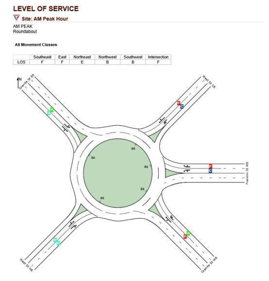
Level of Service (LOS) Method: Delay & v/c (HCM 2010). Roundabout LOS Method: Same as Sign Control.
