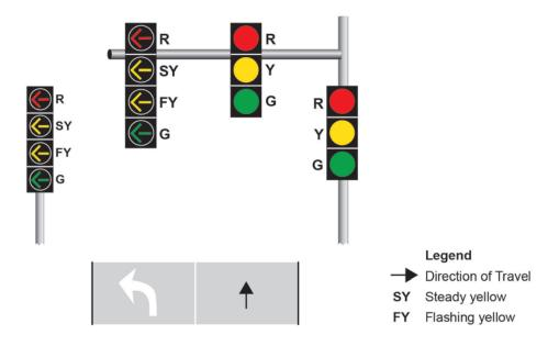
FIGURE 10 Proposed Signal Faces for the Westbound Right-Turn Operation
