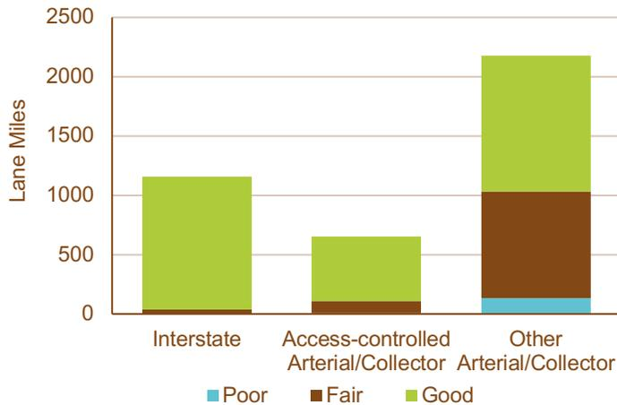
Note: This chart reflects data recorded in the 2014 year-end Massachusetts Road Inventory file, which includes pavement data collected primarily in 2013. *Good*, *fair*, and *poor* classifications are based on IRI ratings. This chart displays data for the 97 municipalities in the Boston region. Source: MassDOT Pavement Management Program.
