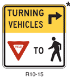
FIGURE 9 “Turning Vehicles Yield to Pedestrians” Sign
