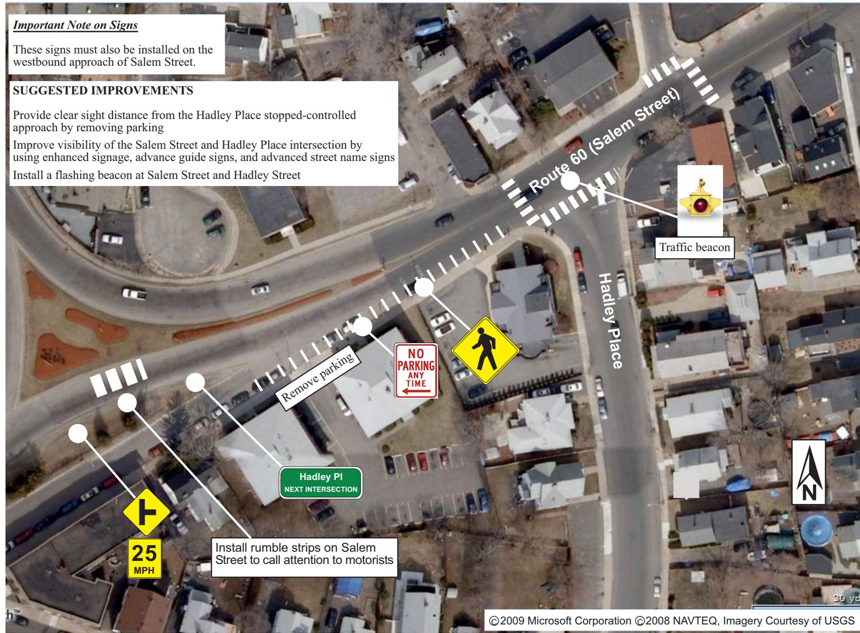
facing the Hadley Place stop-controlled approach and yellow flashers facing the Salem Street uncontrolled approaches. Use of flashing beacons increases the visibility of intersections for approaching drivers, thus supplementing the signage and marking improvements and calling attention to stop signs.
