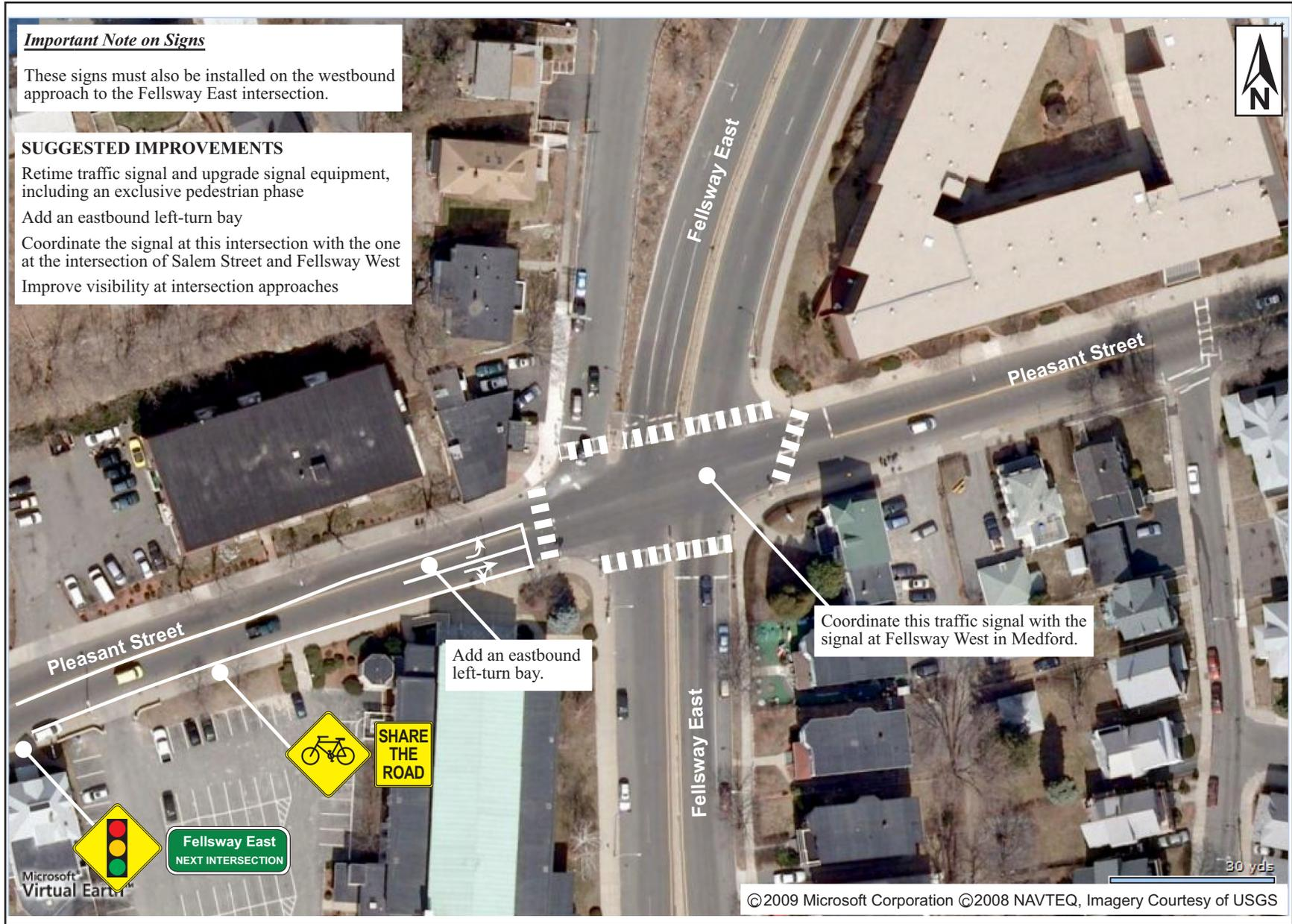
2. Optimization of the signal timing for each phase to minimize delays at the intersection.
