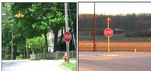
Standard overhead flashing beacon
