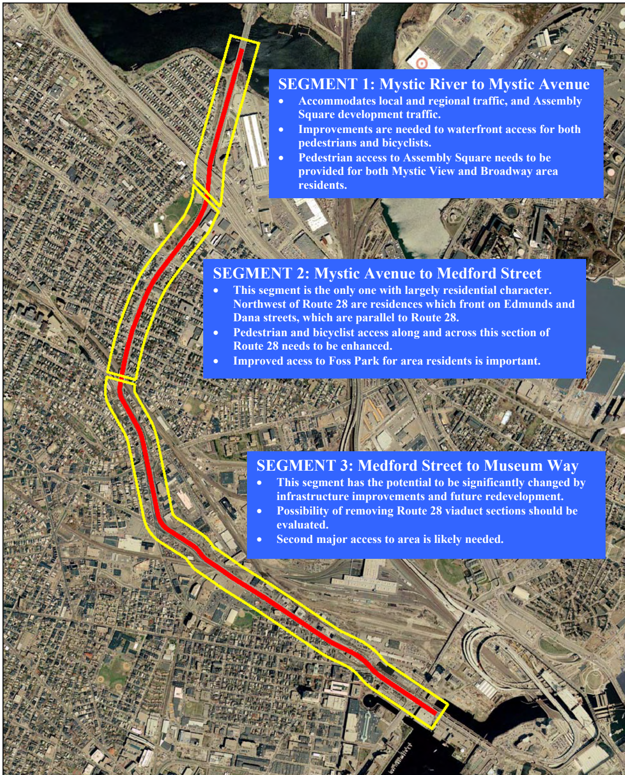
FIGURE 8.1 Corridor Segments and Key Characteristics and Issues
