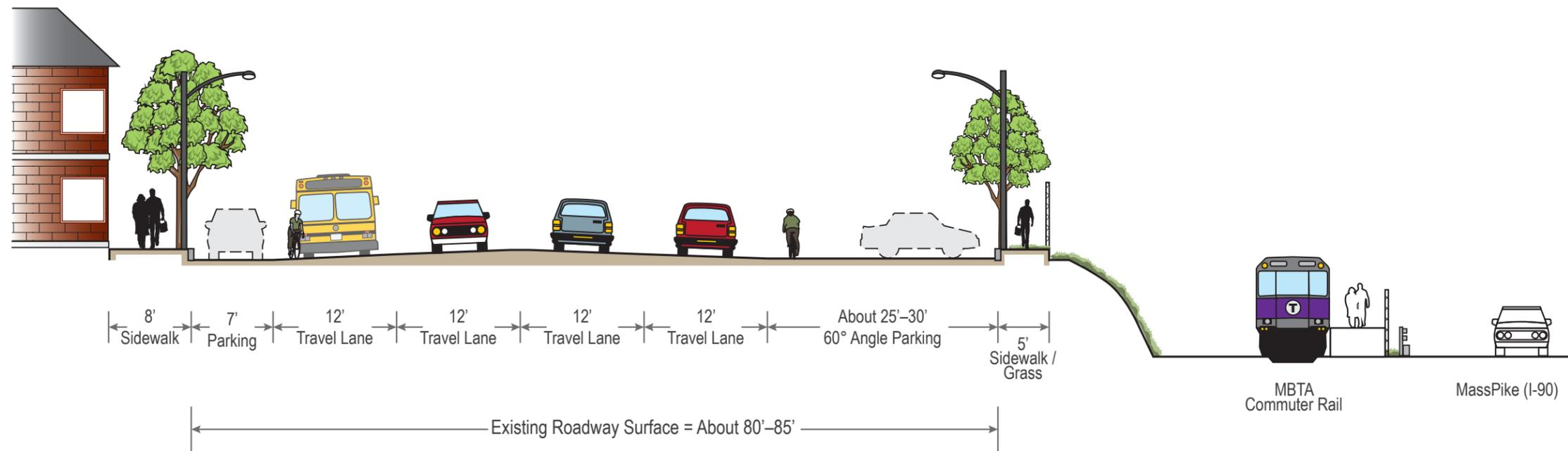
**Roadway Cross-Section in the Newtonville Station Area**
